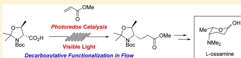
**ABSTRACT:** A formal total synthesis of L-ossamine was achieved. The key feature of the synthesis was the decarboxylative functionalization of a threonine derivative using visible-light-mediated photoredox catalysis. This reaction was implemented in a flow reactor, allowing for the efficient conversion to the desired product.
