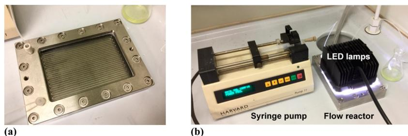
**Figure 2.** (a) Flow reactor for photoreactions (2 mm width, 0.5 mm depth, 3 m length, MiChS Co., Ltd.). (b) Flow reactor setup for the visible-light-mediated decarboxylative functionalization.
