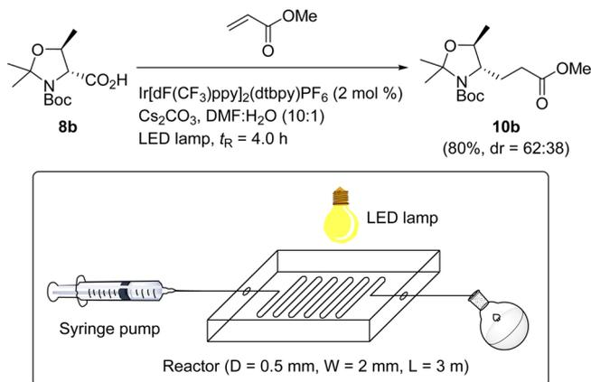
residence time under irradiation of a 48 W LED lamp using a 3 mL reactor provided full conversion of the starting material to the desired product **10b** in 80% yield (50% yield in 47 h in batch, Table 2, entry 5). Using the photo flow reactor could allow the enhancement of irradiation per unit volume to have significant effects on the photoredox reaction course.
