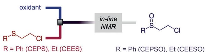
**Scheme 2.** An integrated flow system with in-line NMR monitoring for the sulfoxidation of mustard simulants chloroethyl phenyl sulfide (CEPS) and chloroethyl ethyl sulfide (CEES).
