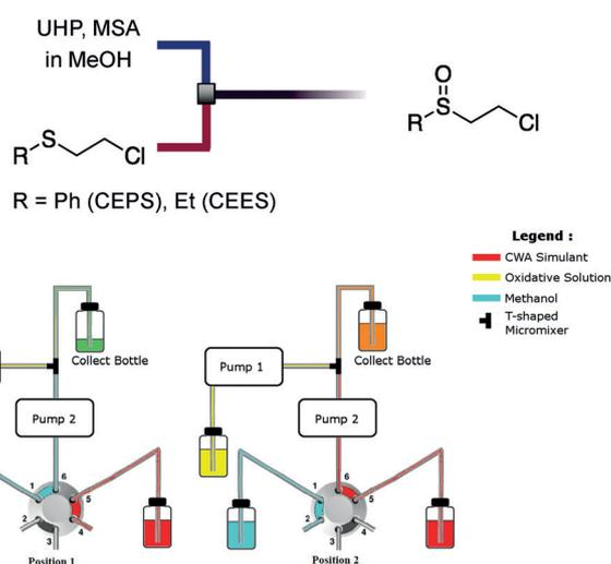
**Figure 1.** Continuous flow set-up for the oxidation of half-mustards CEPS and CEES with UHP/MSA in methanol. See the Supporting Information for details.
