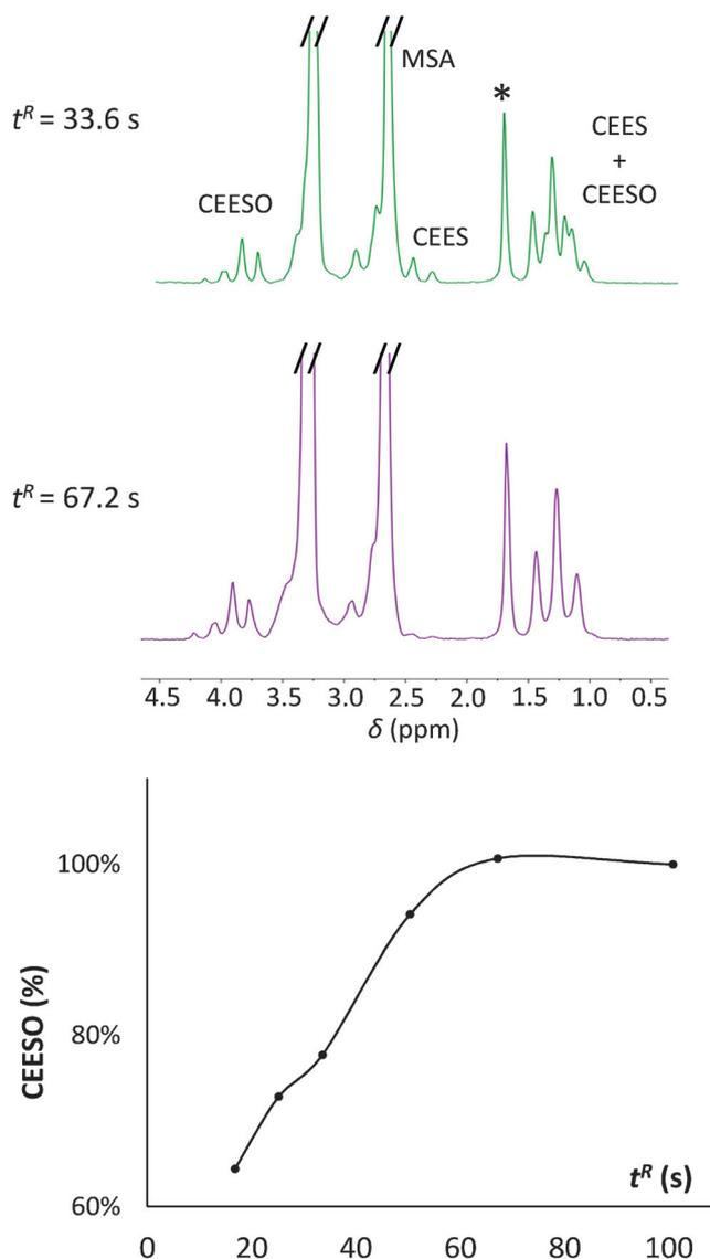
**Figure 3.** Neutralization of CEES monitored by an in-line NMR system. Top and middle: Two NMR spectra recorded at different  $t^R$ . Note that the peak with a \* corresponds to a  $^{13}\text{C}$  satellite line from the residual solvent signal at 3.3 ppm. Bottom: Percentage of CEESO as a function of the residence time.
