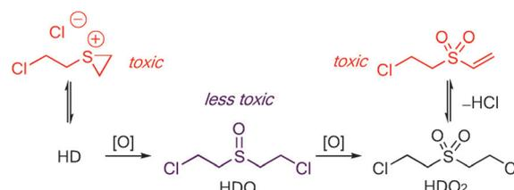
**Scheme 1.** Oxidation of mustard gas yperite (HD) into the corresponding sulfoxide (HDO) and sulfone (HDO<sub>2</sub>).
