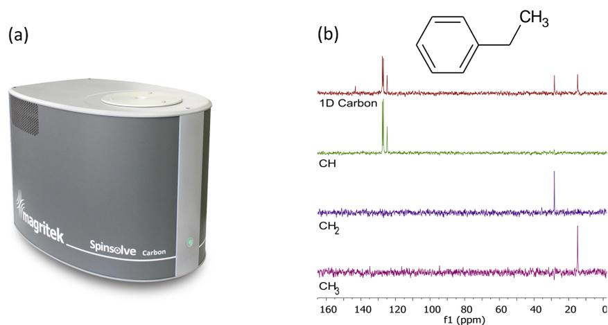
Figure 1: (a) The SpinsolveCarbon benchtop NMR system, (b) carbon-13 spectra of neat ethylbenzene. The spectrum at the top is the full 1D spectrum showing all carbons in the molecule. Spectral editing such as DEPT enable the measurement of subspectra originating from CH, CH<sub>2</sub> and CH<sub>3</sub> groups.
