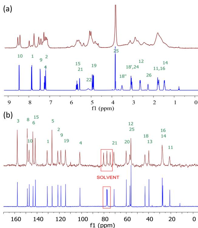
Figure 3: Proton (a) and carbon (b) spectra of the quinine sample measured at 11.7 T (blue) and 1 T (brown). Note that the benchtop proton spectrum shows significant peak overlap due to strong coupling, whilst the benchtop carbon spectrum is essentially identical to the one at high field allowing unambiguous peak assignment [2].
