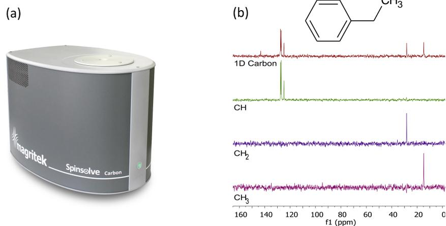
Figure 1: (a) The SpinsolveCarbon benchtop NMR system, (b) carbon-13 spectra of neat ethylbenzene. The spectrum at the top is the full 1D spectrum showing all carbons in the molecule. Spectral editing such as DEPT enable the measurement of subspectra originating from CH, CH<sub>2</sub> and CH<sub>3</sub> groups.
