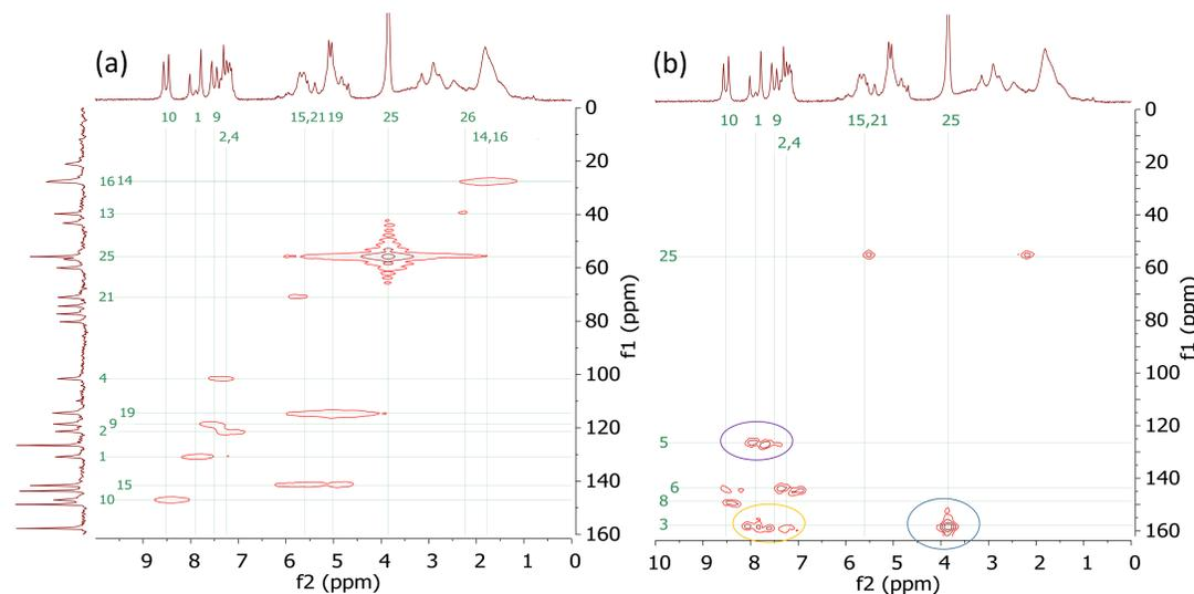
Figure 4: HSQC (a) and HMBC (b) spectrum of quinine at 1 T.
